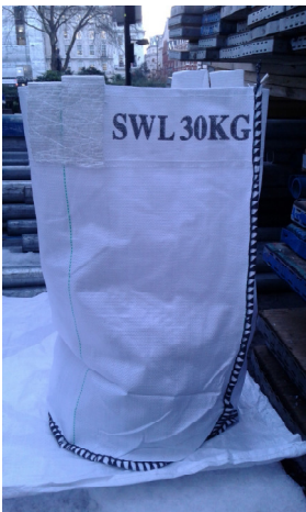
Figure 1 Lifting bag showing SWL
